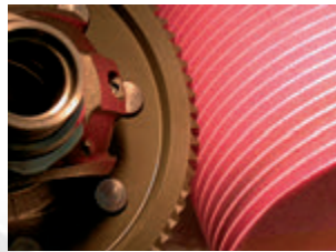
Hermes worm wheels for continuous threaded wheel grinding
